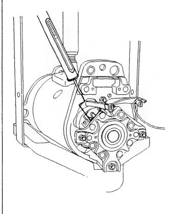
STARTING-MOTOR ASSEMBLY Assembling control relay and starting-motor solenoid Fit control relay and starting-motor solenoid. Use torque wrench. ATTENTION: DANGER OF INJURY Engaging shaft is spring-pretensioned and shoots out of armature on removing starting-motor solenoid. Torque wrench: comm. avail. Tightening torque Hexagon bolts: 11...16 Nm 9,8...14 Nm Securing bolts:
